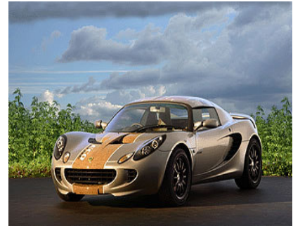
The Lotus Eco-Elise (pictured above) sports body panels manufactured entirely from hemp.
